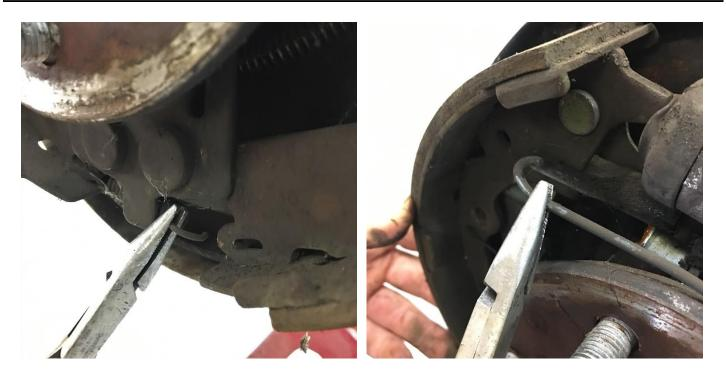
Remove the 2 other retaining springs above and below the axle as shown.
