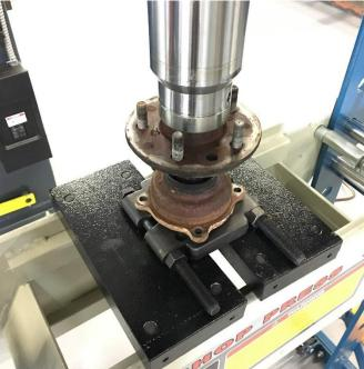
Remove the wheel bearing from the drum backing plate by lightly tapping around the perimeter with a hammer as shown. Optionally, a new wheel bearing can be installed at this time. The axle can now be reinstalled into the bearing on a press by supporting the bearing as close to the center as possible.
