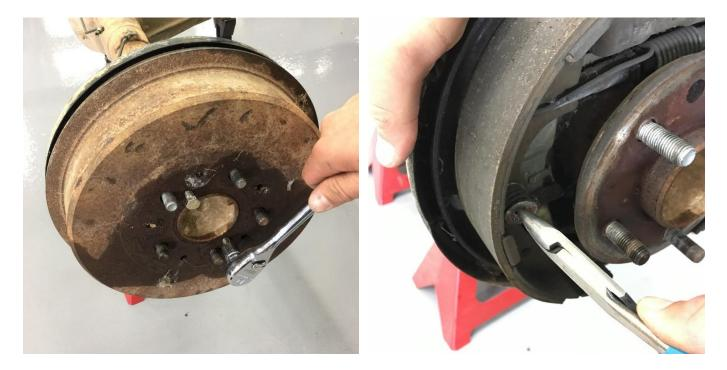
This installation refers to the **passenger side** of the axle. All steps are to be repeated on the driver side. Start by removing the factory drum. It may be necessary use a lubricant around the axle register along with two 5/16-18 bolts threaded into the drum to drive it away from the axle as shown. Once the drum is removed, remove the brake shoe retaining springs (2 places) as shown.
