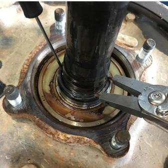
Remove the axle and drum backing plate from the housing. **Steps 10-15 require the use of a press. Refer to Step 16 for removing the backing plate without removing the axle shaft.** Using a pair of snap ring pliers and a small screw driver, open the retaining ring enough to slip it out of the groove and on to the outer diameter of the shaft. Then pull the ring up and off the shaft. Do not attempt to force the ring off of the shaft perpendicularly. It will bend and damage it.
