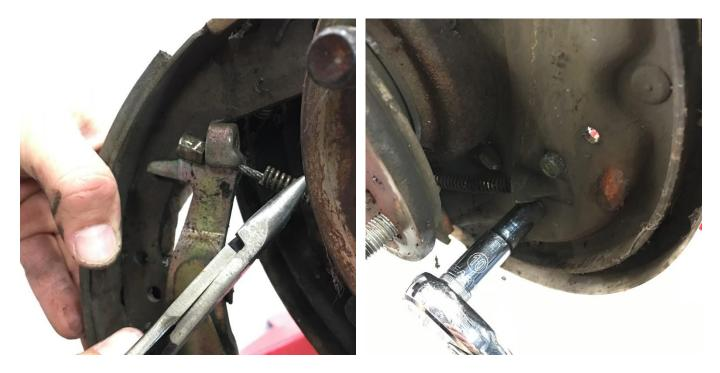
Remove the parking brake cable where it installs into the brake shoe. Then remove the 2 bolts securing it to the drum backing plate. These bolts will need to be kept and reused.
