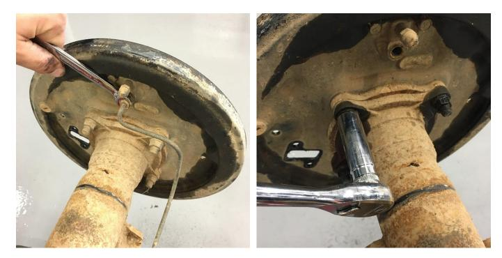
Remove the factory brake line at the back of the drum backing plate. Then remove the 4 bolts securing the axle to the flange. It may be necessary to use a lubricant on these threads.
