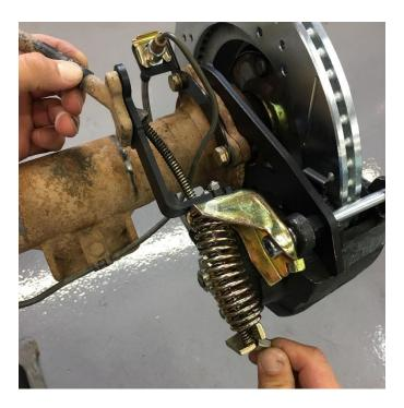
For kits with parking brake calipers, reinstall the factory parking brake cable through the extension bracket and hook to the caliper lever. **NOTE:** Long bed or lifted trucks may require our <u>Parking Brake Cable Kit</u>.
